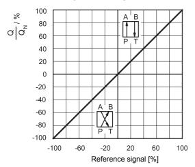
Typical flow rate curves at constant  $\Delta p$  = 70 bar P-T according to the reference signal.
